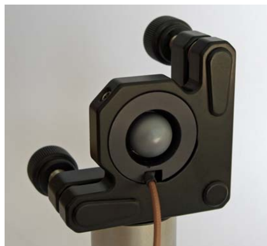
Back view on mounted PCA (THz side)
