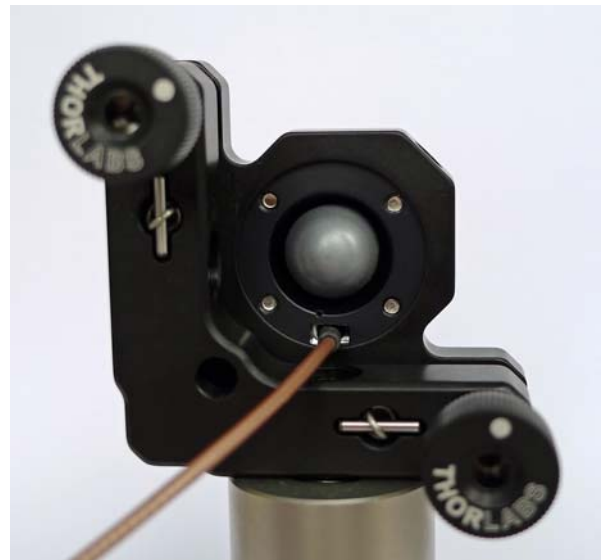
Back view on aspheric silicon substrate lens (THz side)
