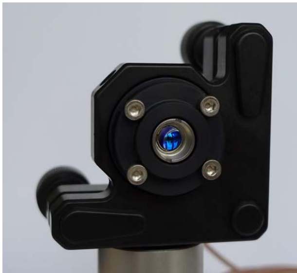
Front view on mounted aspheric optical lens (laser side)
